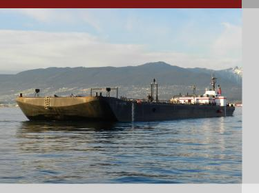
A double-hulled, IMO compliant, OPA 90 oil tank barge. Designed primarily for pushing, the ITB Vancouver is equipped with a powerful omi-directional bow thruster for aiding in docking and maneuvering.
