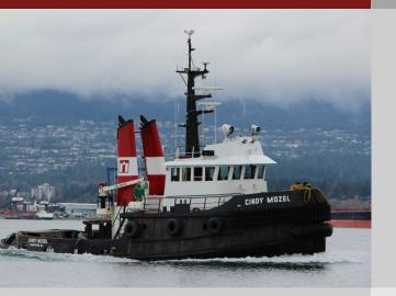
The Cindy Mozel is primarily employed in coastal towing and pushing of Island Tug's oil barge fleet. At 1800 HP and designed for maneuverability, the Cindy Mozel is kept busy with a wide variety of assignments.
