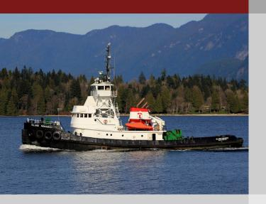
A proven offshore tug of 3000 horsepower, the Monarch is primarily engaged in pushing and towing of Island Tug's large oil barge fleet.
